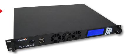
The ATLAS 8000 series platforms are based on a space efficient 1RU rack mount design that can be used to host interface and gateway solutions to inter-connect multiple types of systems through a common IP network. The ATLAS 8000 is available in several variants to meet specific integration needs.
